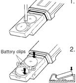
Removing the batteries
